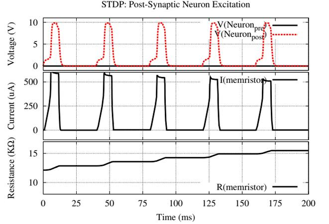
Fig. 6. Simulation: pre-synaptic neuron is suppressed while the post-synaptic neuron is excited; the memristor synaptic weight exhibits an increase in resistance.
