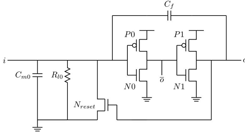
Fig. 2. Leaky-Integrate-and-Fire CMOS Neuron: Classical CMOS neuron firing spikes when its input threshold voltage potential is reached.
