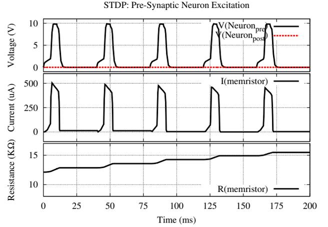
Fig. 5. Simulation: pre-synaptic neuron is excited while the post-synaptic neuron is suppressed; the memristor synaptic weight exhibits an increase in resistance.
