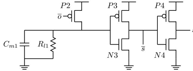
Fig. 3. Neuron Spike Memory: When a neuron fires,  $C_{m1}$  charges up remembering its excitation,  $R_{l1}$  slowly leaks away the charge and thus determining the memory spike retention time.
