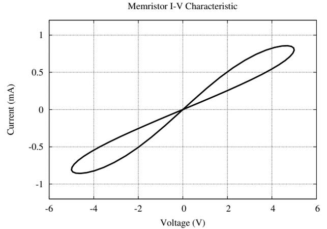
Fig. 1. Memristor Hysteresis I-V Characteristic.
