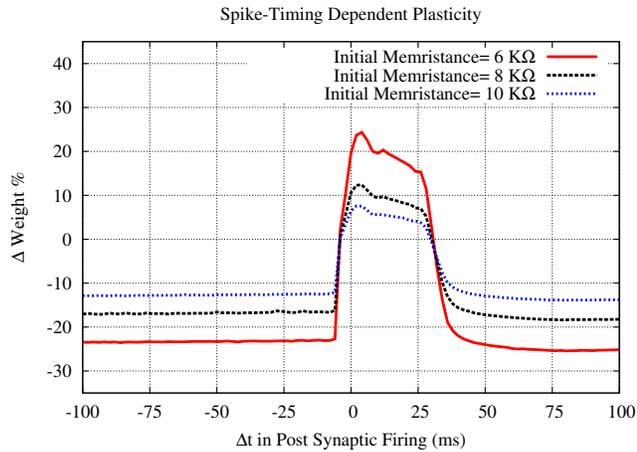
Fig. 7. Simulation: both the pre-synaptic and post-synaptic neurons are excited; the memristor synaptic weight exhibits an increase or decrease in its weight (conductance) dependent on the relative spike timing  $\Delta t$ .
