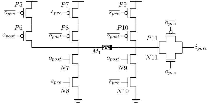
Fig. 4. Synaptic Control Circuit: The  $M_1$  memristor's current flow is regulated based on the spike timings of the pre-synaptic and post-synaptic neurons.
